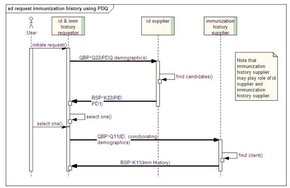
Figure B-49—Sequence Diagram- Request Immunization History using PDQ
