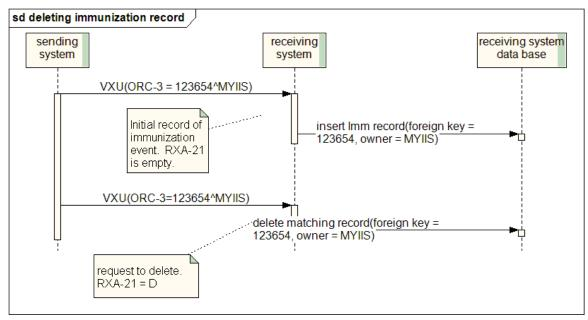
Figure B-46 Sequence Diagram-Deleting an Immunization Record
